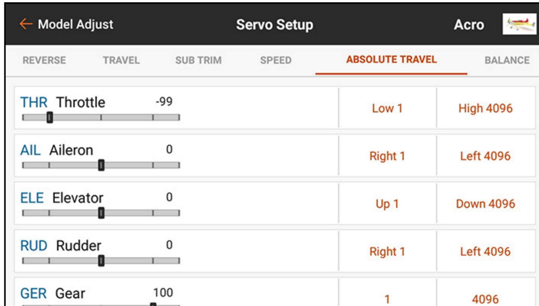
The screenshot shows the 'Servo Setup' menu with the 'ABSOLUTE TRAVEL' tab selected. The menu is titled 'Model Adjust' and 'Acro'. The 'ABSOLUTE TRAVEL' tab is highlighted with a red underline. The following table summarizes the settings for each servo channel:
