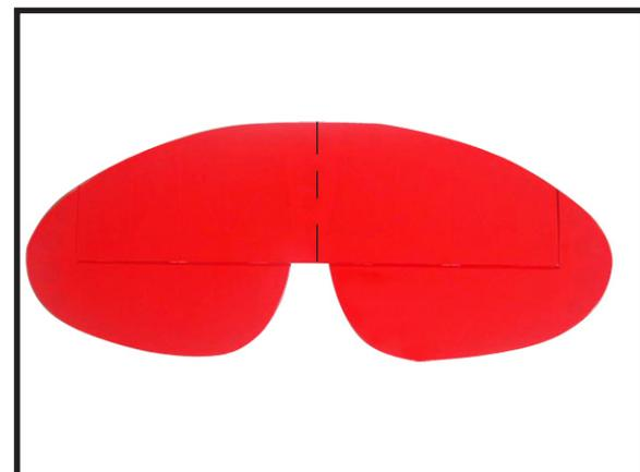
□ 2) Using a modeling knife, carefully remove the covering at mounting slot of horizontal stabilizer ( both side of fuselage).
