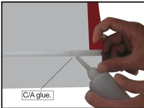
□ 5) Turn the wing panel over and deflect the flap in the opposite direction from the opposite side. Apply thin C/A glue to each hinge, making sure that the C/A penetrates into both the flap and wing panel.
