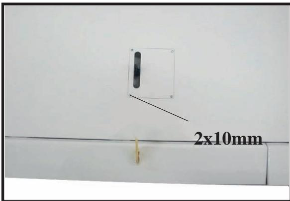
**INSTALLING THE FLAP SERVO**
