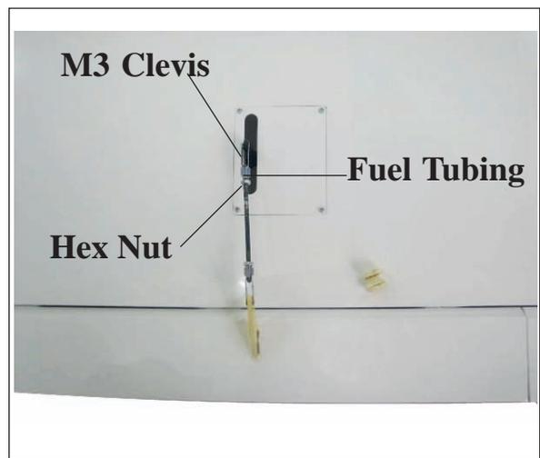
**INSTALLING THE FLAP PUSHROD**
