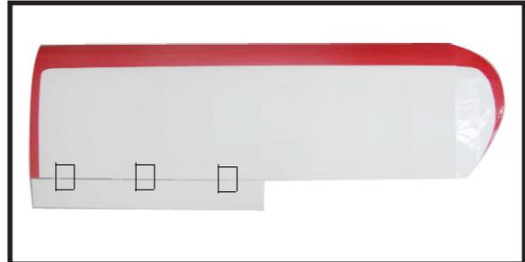
**Note:** *Work the flap down several times to "work in" the hinges and check for proper movement.*
