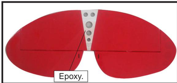
□ 7) When you are sure that everything is aligned correctly, mix up a generous amount of 30 Minute Epoxy. Apply a thin layer to the top and bottom of the stabilizer mounting area and to the stabilizer mounting platform sides in the fuselage. Slide the stabilizer in place and realign. Double check all of your measurements once more before the epoxy cures. Hold the stabilizer in place with T-pins or masking tape and remove any excess epoxy using a paper towel and rubbing alcohol.
