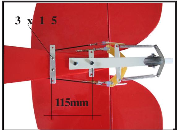
**INSTALLING TAIL STRUTS SUPPORT.**
