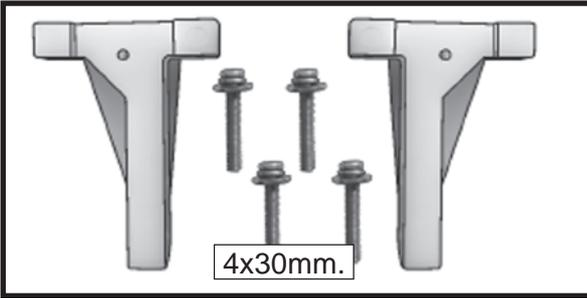
2) Use four 4x30mm head bolts and four 4mm washers to attach the engine mount rails to the firewall. Tighten the screws . Make sure to use threadlock on the screws to help prevent them from vibrating loose.
