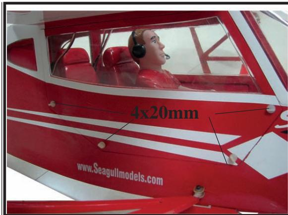
**INSTALLATION STRUT WING-FUSELAGE.**
