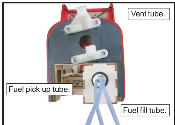
9) Connect the lines from the tank to the engine and muffler. The vent line will connect to the muffler and the line from the clunk to the carburetor.
