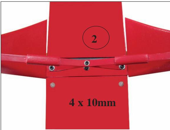
**INSTALLING WHEEL PANTS TO MAIN LANDING GEAR.**
