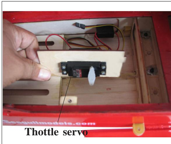
**THROTTLE SERVO ARM INSTALLATION.**
