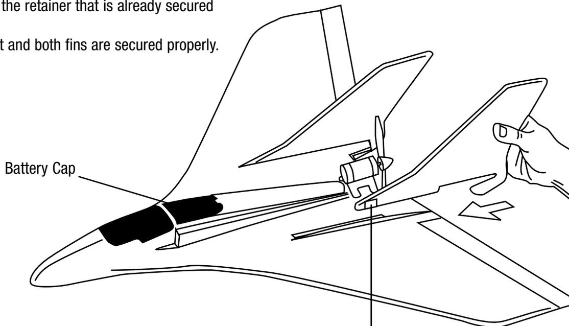
**Note:** It may be helpful to add a few drops of CA to the front tips of the vertical stabs in order to keep them in place while flying your F-27C Stryker PNP. There is rubber double-sided tape on the front of each one, but over time, and despite a tight tension fit when you slide the fins on the first time, they can lose their sticking power. At speeds exceeding 80 mph, it is good, for your safety and the safety of your plane, to add CA to ensure they will stay in place.
