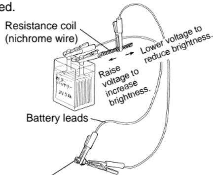
Adjust applied voltage by changing the position of clip on resistance coil until glowplug element is glowing bright red.
