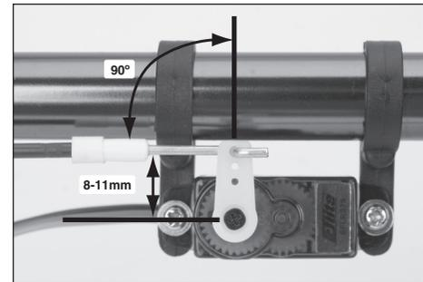
After installing the tail rotor pushrod linkage on the tail servo arm, and ensuring the tail servo is still centered electronically, adjust the length of the pushrod so the tail pitch slider is centered on the tail rotor shaft, between the tail case and tail hub.
