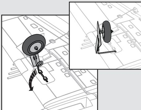
2. Pull the landing gear strut out of the mounting plate hole.
