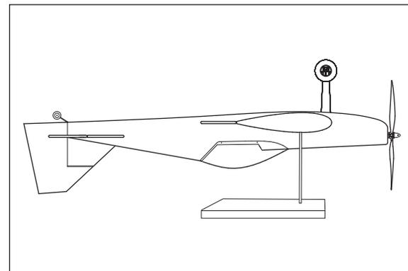
Adjust the motor battery as necessary so the model is level or slightly nose down. You should find the CG to be very close with the battery installed as shown in this manual. Mark the location of the battery on the battery tray using a felt-tipped pen so it can be returned to this position if it is removed from your model.
