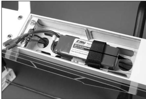
Once you model is balanced correctly, it is recommended to mark the position of the battery in the battery compartment using a pencil or felt-tipped pen. This way it can be returned to the same location after it has been removed for charging.
