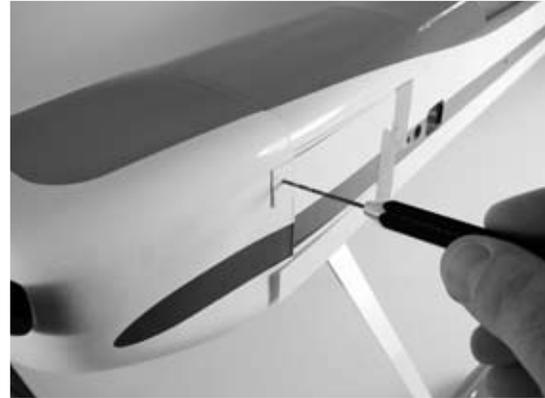
6. Enlarge the holes in the cowl using a  $5/64$ " (2mm) drill bit. Secure the cowl using four 2mm x 8mm sheet metal screws. Snap the spinner cone onto the spinner backplate once the cowl is secure.
