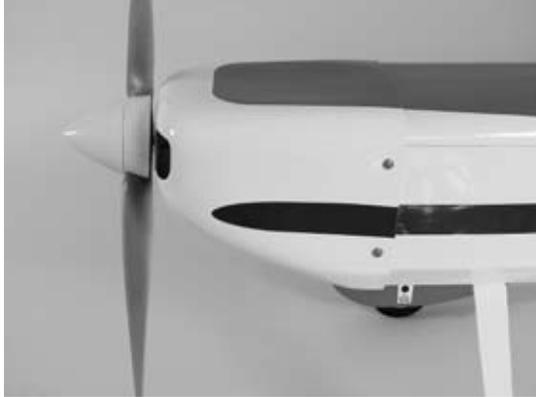
**Hint:** Use thin CA to harden the holes drilled into the cowl mounting tabs. This will help to prevent the screws from vibrating loose in flight.
