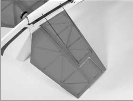
**Note:** Make sure the rods are positioned so they don't interfere with the operation of the rudder and elevator linkages.
