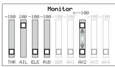
This example of the channel monitor shows the stick positions for assigning a switch, the switch selection on Aux2, and +/- 100% travel on the switch.
