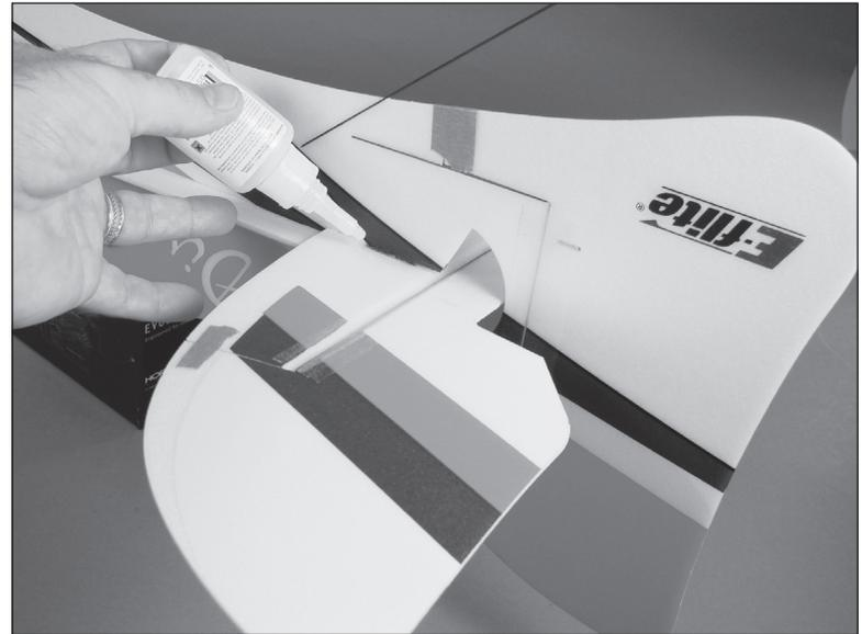
Hint: Use low-tack masking tape to hold the fin/rudder and stabilizer/elevator in neutral. This will make the assembly of your airframe slightly easier than if they are moving about while handling the airframe.
