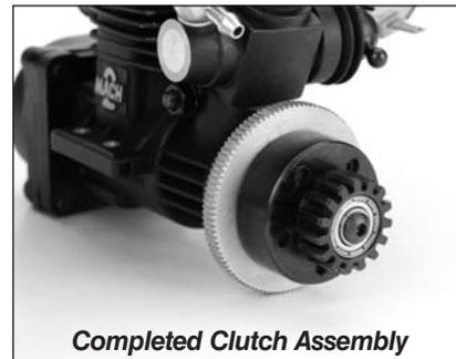
Final end play for the clutch bell is adjusted with the 5 x 7 shims. Use enough shims to allow approximately .5mm of endplay on the clutch bell. If the endplay is larger than .5mm add 5X7 washers to the outside of the clutch bell in order to remove excess play. When the assembly is finished the clutch bell should be able to spin freely with no drag. If there is excess drag, check the clutch bell bearings for smooth operation or remove a shim from behind the 3 x 6 button head screw.
