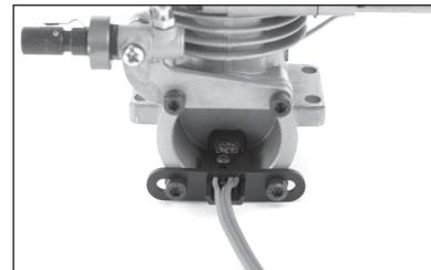
**Note:** On some engines you may need to space the sensor further away from the backplate. The sensor picks up the crankpin only; on some engines if the sensor is too close, it will not distinguish the crankpin from the crank weight.
