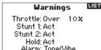
Highlight the desired warning (Throttle, Stunt 1, Stunt 2 or Hold or Throttle, Flaps, Gear, Flight Mode 1 and Flight Mode 2 for airplane model) then press the roller to select. Now rotate the roller to inhibit or activate the selected warning.
