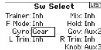
Select the channel or function you wish to assign. See chart for options. Press the roller to accept. Note that a channel or function can only be assigned once. Repeat to select all desired switch positions.
