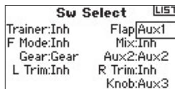
Rotate the roller to select the desired channel or function you wish the switch, knob or trimmer to operate. Press the roller to accept. Note that the channel or function can only be assigned once.
