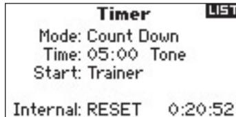
Select Inhibit, Count Down or Stop Watch. Press the roller to accept.
