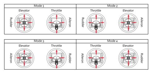
Changing from modes 2/4 to 1/3 will change the throttle position. This will require the user to open the system and switch the stick positions. The gimbals can be switched by following these instructions.
