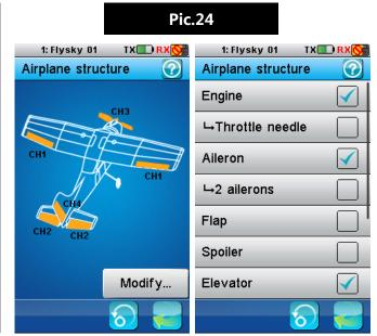
The system automatically adjusts the menu in accordance with the contents of the aircraft structure and will hide unrelated functions. If you wish to use a feature, but cannot find the relevant menu, refer to the table below to make sure the correct control surfaces have been added to your model.
