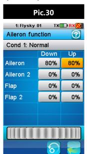
This function can also mix aileron movement to flaps and elevators.
