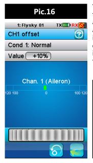
This function can be used to correct problems with alignment. For example if a servos range of motion is too great in one direction and not enough in another, it is possible to offset the channel by +/- 50%.
