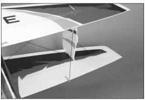
25. Apply a drop of foam-safe A to the heat shrink at both the top and bottom ailerons. Make sure to apply CA to both the pushrod and control horn.
