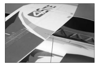
QQ 24. Use side cutters to trim the carbon rod to the proper length. Use a piece of heat shrink and a soldering iron to make the connection between the top and bottom ailerons.
