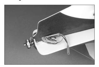
8. Check the operation of the motor at this time. It should rotate counterclockwise when viewed from the front of the aircraft. If not, follow the instructions provided with your speed control to correct the situation.
