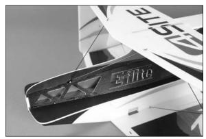
7. Check the alignment between the wings and stabilizer. Position the stabilizer so it is parallel to both the top and bottom wings as shown. It should also be square to the fuselage. Check to make sure that the wing and stabilizer are also perpendicular to the fuselage.
