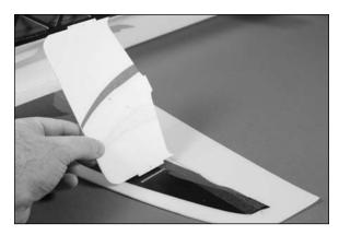
OO 6. After confirming the fit between the outer strut and bottom wing, use foam-safe CA to glue the outer strut to the wing. Use a square between the outer strut and bottom wing to keep them in alignment while the CA fully cures.
