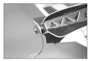
7. Pass the motor wires through the slot in the front of the fuselage. Connect the wires from the motor to those of the speed control. The battery lead from the speed control can now be passed to the opposite side of the fuselage through the slot in the fuselage as well.
