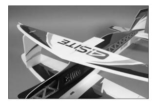
10. Remove the top wing and place it upside down on your flat work surface. Use foam-safe CA to glue the top wing to the fuselage and outer struts. Make sure to use a square at both the struts and fuselage to keep things in alignment while the CA cures.
