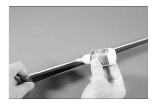
4. Position the horizontal fuselage on the main fuselage, again making sure that they line up at the front. Use a square at multiple points on the fuselage from nose to tail to guarantee the horizontal fuselage is square to the main fuselage. Check square from both the top and bottom side of the fuselage. Allow the CA to fully cure before proceeding.
