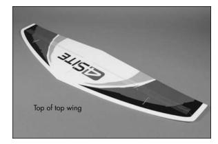
9. Test fit the top wing to the fuselage and outer struts. The tab on the struts and fuselage will be flat in the top wing. If not, it may induce an unwanted airfoil that could result in unwanted flight characteristics.
