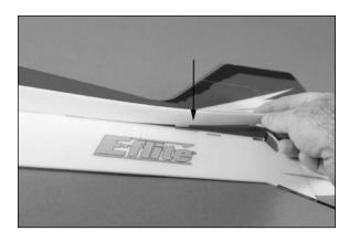
3. Remove the horizontal fuselage from the main fuselage. Apply a bead of foam-safe CA to the left horizontal fuselage where it contact the main fuselage. Do not apply CA to the rear section of the horizontal fuselage as noted in the previous step.
