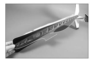
O 10. Locate the Depron firewall. Note the alignment points on the firewall and how they relate to fuselage. The alignment points are located on the top and left (as viewed from the front of the fuselage) as up and right thrust are built into your model. Use foam-safe CA to install the Depron firewall in the fuselage.
