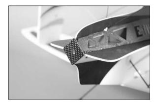
4. It may be necessary to remove a small amount of material from behind the firewall to clear the motor shaft of your particular motor. You can use either a round file or hobby knife to accomplish this task.
