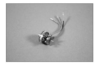
O 6. Use a #1 Phillips screwdriver and the two screws provided with your motor to attach it to the firewall. Work slowly to avoid applying too much pressure, resulting in damage to your airframe.
