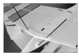
4. Test the fit of the two wheel skids on the ends of the carbon rods. The skids will be parallel to the fuselage when installed correctly. Use thin CA to glue the skids to the carbon rods.
