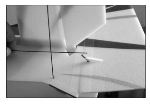
12. The pushrod is supplied slightly long to accommodate for servo selection and control horn position. Use side cutters to trim the pushrod so it almost touches the rudder control horn.
