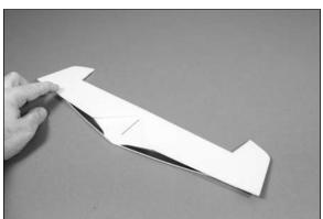
8. Slide the folded horizontal stabilizer into the fuselage. Unfold the elevator and position the stabilizer, but do not apply any glue to the stabilizer at this time.
