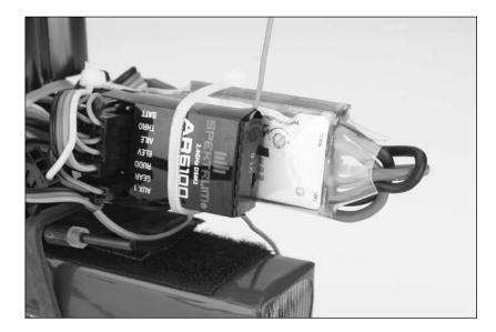
Once the receiver is mounted securely, route the antenna(s) per the instructions included with the receiver. In
