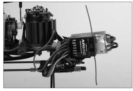
If using a 72MHz receiver, you can route the antenna around the landing gear and be certain to secure any excess length of the antenna to prevent it from coming into contact with any moving parts on the helicopter.
