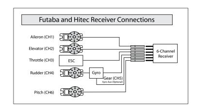
• After connecting the wire leads to the receiver, remove the remaining paper backing from the two-sided tape on the receiver. Then, carefully straighten the antenna(s) and place the receiver onto the front tray. Fasten the receiver in place on the front tray and use one of the included zip/cable ties for added security. However, be sure not to tighten the zip/cable tie too much as it could damage the case of the receiver.
