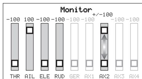
This example of the channel monitor shows the stick positions for assigning a switch, the switch selection on Aux2, and +/- 100% travel on the switch.
