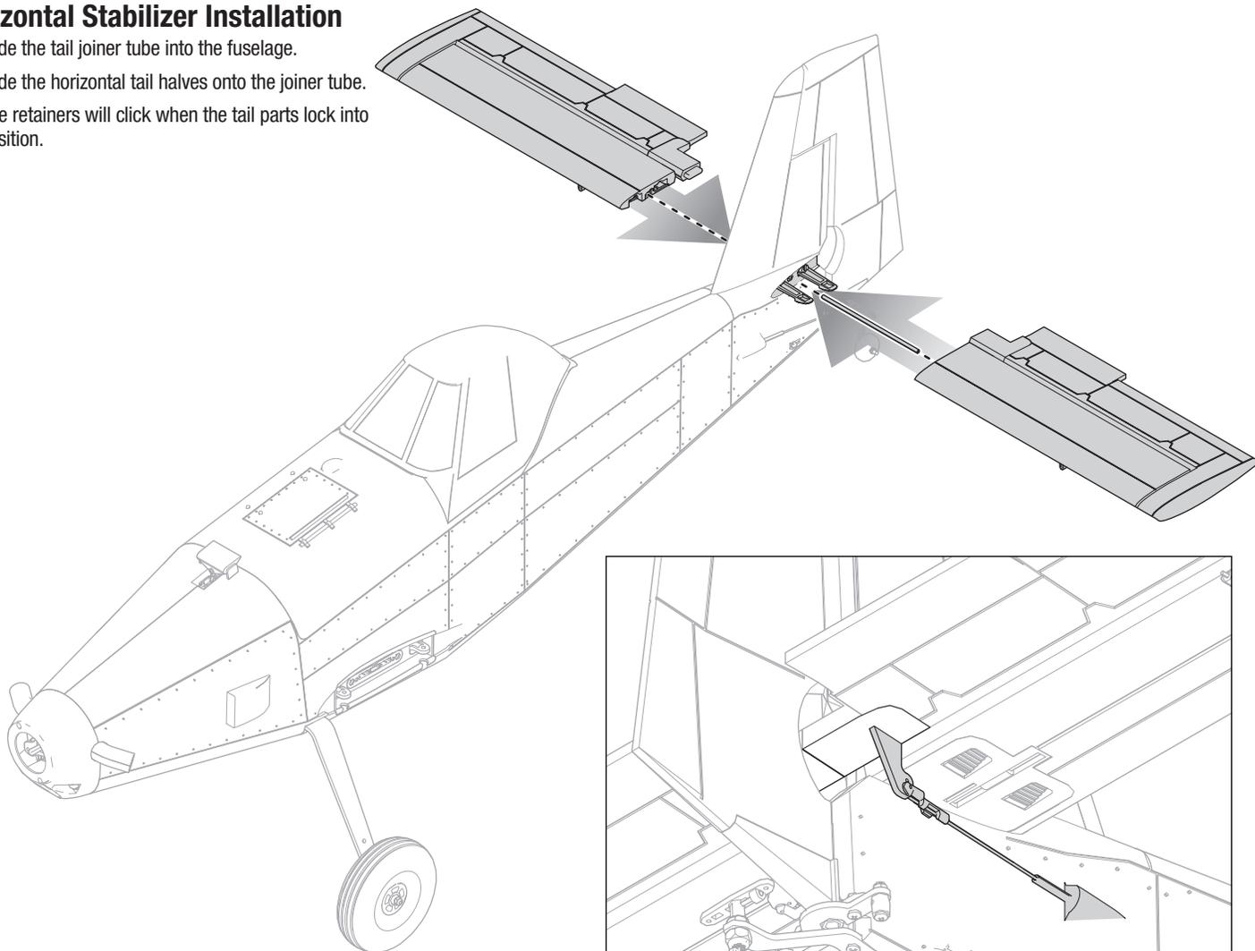
4. Insert the elevator pushrod into the outside hole on the elevator control horn.
