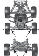
\*Front arms inner and outer hinge pins should be in a imaginary horizontal line when ride height is set
