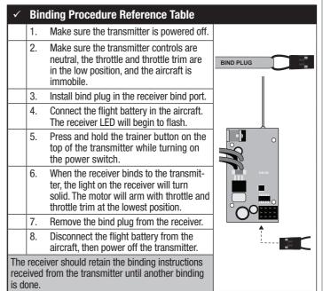
\*The throttle will not arm if the transmitter's throttle control is not put at the lowest position. If you encounter problems, follow the binding instructions and refer to the transmitter troubleshooting guide for other instructions. If needed, contact the appropriate Horizon Product Support office.
