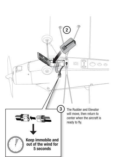
The aircraft can be held immobile for 5 seconds at any angle convenient for you to connect the battery.
