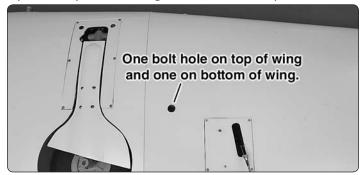
☐ 5. Once the epoxy has cured, slide the wing panels together completely. Locate and cut the covering from over the two outer wing panel bolt holes, one on top and one on bottom.
