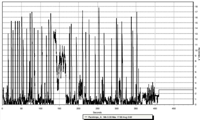
In the example above, the average current was 2.62 amps, which calculates to 435mAh per 10 minutes (typical flight length). It's recommended that only 60% of the available capacity be used to ensure plenty of reserve battery capacity. In this example, using two 4000mAh batteries (8000mAh total capacity) x 60% = 4800mAh (available usable capacity) divided by the capacity used per 10-minute flight. 435mAh would allow up to 11 flights of 10 minutes each.
