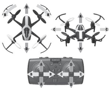
**Basic Flight** Advance the throttle slowly until your Kodo HD rises into the air. The controls are very sensitive and small stick movements should be used to the control the quadcopter. If you get into trouble and see that the Kodo HD is going to crash, move the throttle to its lowest position immediately.
