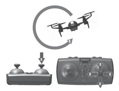
**Flips** Push down on the right stick and release it when the controller beeps. Move the right stick in any direction and release it when the Kodo starts to flip.
