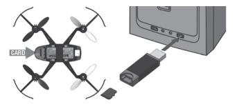
Only insert and remove the memory card when the battery is not connected to the Kodo HD. When the memory card is installed, there will be a steady blue LED just above the card slot.
