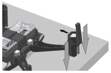
1. Remove the rotor blade from the motor.
