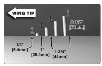
☐ 10. Clean the aluminum tubes with denatured alcohol and glue the gun barrels in the wing with
