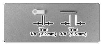
☐ 17. Trim approximately 1/8" (3.2 mm) from the end of the nylon ball socket before threading the 2-56 x 1" (25.4 mm) threaded rod into the end. Also trim 3/8" (9.5 mm) from the end of the threaded rod.
