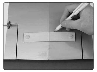
☐ 1. Place the wing bolt plate on the bottom of the wing and insert the 1/4-20 x 2" [51mm] nylon wing bolts through the wing bolt plate and the wing. Mark the outline of the wing bolt plate onto the bottom of the wing.
