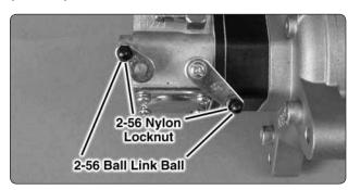
☐ 4. Install a 2-56 ball link ball on the throttle arm and on the choke arm and secure them with 2-56 nylon locknuts. Also remove the throttle arm and position
