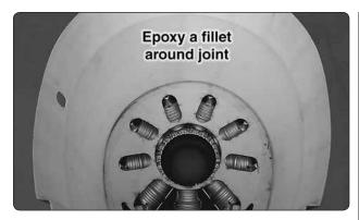
☐ 14. Before gluing, use sandpaper to roughen the gluing area inside the cowl. Clean the area with a paper towel dampened with denatured alcohol. Mix approximately 1/2 oz [14.7cc] of 30-minute epoxy. For a stronger joint, add some milled fiberglass to the epoxy. Apply epoxy to the edge of the engine assembly and insert it in the cowl. Use the remaining epoxy to create a fillet around the edge of the assembly.
