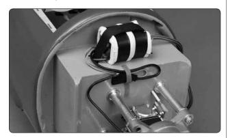
19. Place the ignition module on a piece of R/C foam rubber (not included) and secure it to the top of the firewall box with hook and loop material. The
