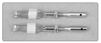
☐ 6. Thread a 4-40 nut and a 4-40 metal clevis, 12 turns, on to each of the 4-40 rigging couplers. Slide a silicone clevis retainer over each clevis. Install the clevises on the tailwheel steering servo arm in the holes 7/16" [11.1mm] from the center of the servo arm.
