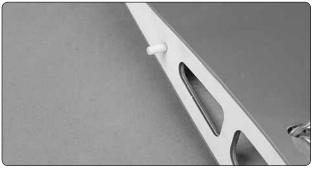
□ 3. Use 6-minute epoxy to glue the two 3/8" [9.5mm] diameter forward wing dowels in the leading edge of the wing. The wing dowels should protrude approximately 1/2" [12.7mm] from the wing. Also glue the 1/4" [6.4mm] aft root rib guide dowel in the left wing half. Clean off any excess epoxy before it cures.
