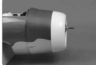
☐ 16. Test fit the cowl over the engine. Install the recommended propeller on the engine. Adjust the position of the cowl so that the dummy radial engine is centered on the drive washer and the propeller clears the front of the cowl by 1/8" [3.2mm]. The cowl mounting brackets should be approximately 1/8" [3.2mm] inside the edge of the cowl.
