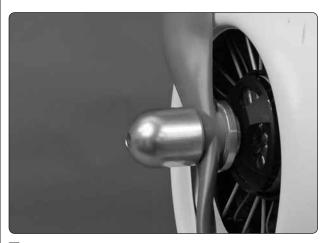
☐ 5. Secure the spinner cone to the spinner adapter with a 10-32 x 1" socket head cap screw (not included).
