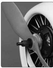
□ 4. APC Electric Propeller: Enlarge the propeller shaft hole to 10mm using a metric prop reamer or a size 'X' drill bit. Trim 1/4" [5 mm] from the end of the spinner adapter (GPMQ4590 not included) so that the adapter is 1-1/4" [32 mm] long. Install the propeller on the motor shaft and secure it with the spinner adapter and washer.
