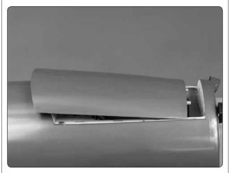
☐ 1. The removable battery hatch is secured at the factory with four #2 x 3/8" (9.5 mm) sheet metal screws. Remove the four screws from the inside of the fuselage. Using a sharp knife blade, locate and carefully cut the battery hatch from the fuselage. Extra Olive Drab covering has been provided to cover the edges of the hatch and the fuselage along the cut.
