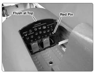
□ 5. Insert one of the red round headed pins in the lower right corner of the instrument panel to represent a knob. Glue the instrument panel in the front of the cockpit so that the top of the instrument panel is flush with the top of the fuselage. Canopy glue or thick CA works well for attaching the instrument panel.
