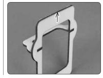
a. Glue the forward fuel tank stop to the forward fuel tank support. Make sure the embossed arrow is on the opposite side of the fuel tank stop.
