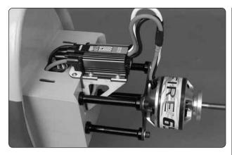
9. Attach the ESC to the ESC mount with four #4 x ½" sheet metal screws and #4 flat washers.
