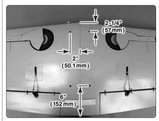
☐ 7. Trim the covering from over the four corresponding holes in the bottom of the wing.
