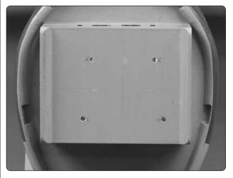
☐ 2. Drill a 13/64" (5 mm) hole through the firewall at each of the appropriate locations marked with an "X" or "+".
