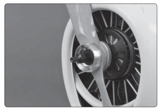
☐ 6. **Xoar Electric Propeller**: Enlarge the propeller shaft hole to 10mm using a metric prop reamer or a size 'X' drill bit. Secure the propeller and spinner base with the spinner adapter and washer (GPMQ4590) (not included).
