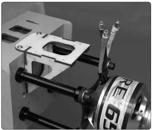
$\square$  8. Position the ESC mount on the firewall box and drill four 5/64" (2 mm) pilot holes through the firewall box. (Two on top and two in the front.) Attach the ESC mount with #4 x ½" (12.7 mm) sheet metal screws and #4 flat washers. Harden the screw holes with thin CA.
