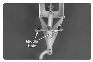
4. Enlarge the middle hole in both sides of the steering arm with a 3/32" [2.4mm] drill. Insert a 2-56 ball link ball in the hole. Secure each ball with a 2-56 nut and a drop of threadlocker.
