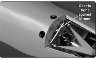
☐ 11. Drill four 3/32" [2.4mm] holes through the rails for mounting the tail gear. If your drill bit is not long enough to reach the rail nearest the top of the fuselage, use medium CA to temporarily glue a 3/32" [2.4mm] drill bit in a 1/8" [3.2mm] brass tube. After drilling the holes, the drill bit can be removed from the tube by heating the tube.
