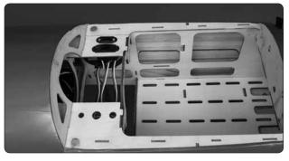
4. Mount the receiver on/off switch and the charge receptacle in the tray under the battery hatch.
