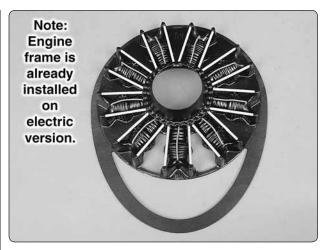
☐ 12. The plywood engine frame can be painted black. Use 6-minute epoxy to glue the plastic radial engine to the plywood engine frame. Align the radial engine with the embossed circle on the plywood frame.
