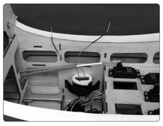
☐ 13. Glue the plywood pushrod support so that the pushrod is inline with the servo arm and on the outside of the aft fuel tank support.
