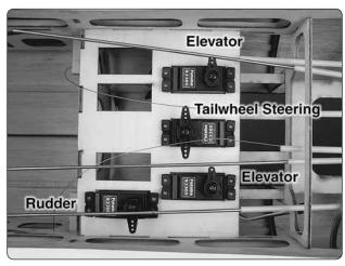
4. Place two elevator, one rudder and one tailwheel steering servo in the servo tray as shown. Make three one-arm servo arms and one two-arm servo arm from the servo arms that came with your servos. Center the servo arms and the trim on your transmitter.
