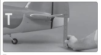
2. Measure the high rate elevator throw first. Move the elevator up with your transmitter and move the
