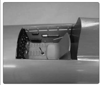
☐ 7. Trim the seat along the cutout lines and glue it to the pedestal on the cockpit floor. Now glue the control stick in the previously drilled hole using the height of the seat as a guide.
