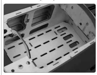
☐ 2. Insert the tabs on the front of the battery tray in the firewall. Note that the front of the battery tray is angled to match the right thrust built into the firewall. Check that the tray is seated on the formers and then securely glue it in the fuselage.
