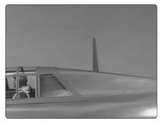
9. Insert the antenna mast in the top of the fuselage. The mast is held in place with magnets.
