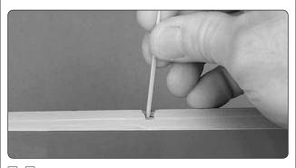
□ 7. Mix up approximately 1/4 oz. [7.4cc] of 30-minute epoxy. Use a toothpick to thoroughly apply the epoxy in the holes in the fin and rudder. Use the toothpick to get the epoxy out of the opening of the holes in the rudder and fin so it doesn't get into the hinge pin. Wipe away any excess epoxy around the outside of the holes with a couple of the small paper towel squares dampened with denatured alcohol.
