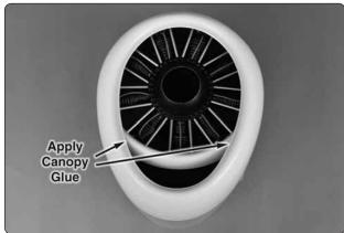
☐ 15. Trim the white turbo charger/oil cooler intake around the base. Then mark and trim the top of the intake 3/8" [9.5mm] from the base. Trial fit the intake
