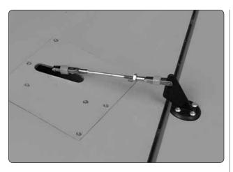
☐ 4. Slide a silicone clevis retainer over the solder clevis. Reinstall the aileron pushrod with the threaded clevis attached to the control horn.
