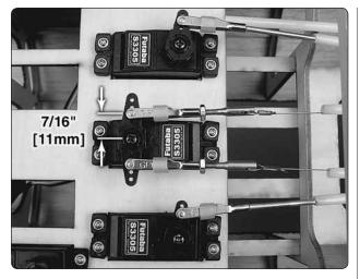
☐ 7. Connect the tailwheel steering servo to the rudder servo with a Y-harness. Center the servo arm and the tailwheel gear. Install a swage on each cable, securing it following the same procedure used on the tail gear. Use a pliers to crimp the swage tightly on the cable.
