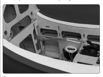
☐ 16. Install the choke servo, 2-56 x 1" (25.4 mm) threaded rod, white inner pushrod tube and nylon clevis following the same procedure used for the throttle pushrod.
