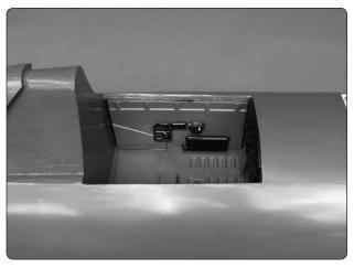
☐ 6. Trim the sides of the cockpit leaving approximately 1/16" [1.6mm] lip around the edges. Apply the decals to the numbered locations on the side cockpit panels. Install the white and red round head pins and decals as shown. The top edge of the cockpit sides should fit under the stringer at the top of the cockpit.
