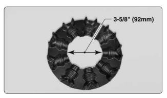
□ 5. The center hole in the radial engine will need to be enlarged to 3-5/8" (92 mm) to fit over the RimFire 65cc electric motor.
