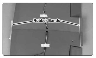
☐ 4. Once the epoxy has cured, remove the clamps from the wing joiner and sand off any excess epoxy you may have missed. Test fit the wing joiner in each wing half making sure that both wings halves fit together at the root without any gap. Trial fit clamping the wing
