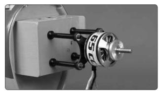
☐ 6. Follow the Stand Off Motor Mount instructions to install the motor on the firewall box. The RimFire 65 motor uses the embossed 'X' pattern on the front of the firewall box. Drill a 5/16" [8mm] hole at each mark.
