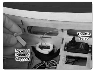
☐ 11. Mount the throttle servo in the servo tray and slide a plywood pushrod support onto the outer pushrod tube.
