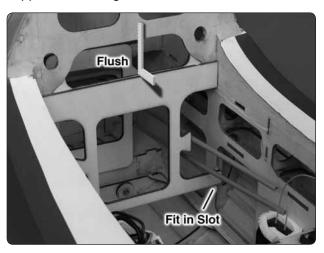
☐ 10. Glue the aft fuel tank support to the #2 former. It should be flush with the edge of the lightening hole and fit into the slots in the fuselage side
