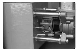
☐ 18. Install the nylon ball socket and threaded rod on the choke following the same procedure used for the throttle pushrod.
