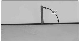
4. Without using any glue, install five hinges into the rudder. Note that the pivot point of each hinge must align with the center of the leading edge. To achieve this alignment, the hinges will be fairly deep in the rudder. Also note that the hinges must be perpendicular to the leading edge.
