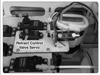
☐ 4. Glue the retract control valve mount on the retract servo tray.
