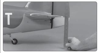
☐ 1. Use a box or something similar to prop up the bottom of the fuselage so the horizontal stabilizer and wing will be level. Hold a ruler vertically on your workbench against the widest part (front to back) of the trailing edge of the elevator. Note the measurement on the ruler.
