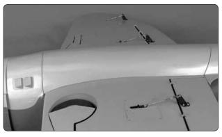
☐ 5. Glue the belly pan to the wing using 30-minute epoxy. Make sure that the belly pan is tight against the bottom of the wing and centered between the fuselage. Wipe off any excess epoxy before it cures.
