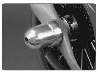
☐ 3. Install the prop hub cone on the engine using a M5 x 50mm socket head cap screw. Use a drop of threadlocker on the threads.
