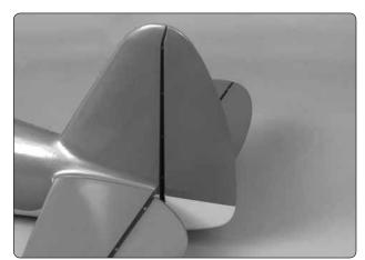
□ □ 5. Again without glue, test fit the rudder to the fin. Move it left and right a few times to align the hinges. The rudder doesn't have to move very far, only 2" [50.8mm] left and 2" [50.8mm] right measured at the widest part of the rudder at the trailing edge. If there
