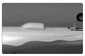
☐ 1. Position the turbocharger exhaust fairing as shown. Mark on the fuselage the outline of the fairing. Inside the outline use a T-pin to prick small holes in the covering, or trim and remove the covering from inside the outline. This will help the glue hold the fairing on. Glue the turbocharger exhaust fairing on the fuselage with canopy glue or medium CA.
