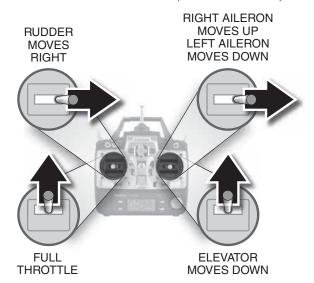
☐ 3. Make certain that the control surfaces and the carburetor respond in the correct direction as shown in the diagram. If any of the controls respond in the wrong direction, use the servo reversing in the transmitter to reverse the servos connected to those controls. Be certain the control surfaces have remained centered. Adjust if necessary.
