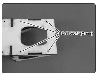
☐ 7. Assemble the ESC mount as shown. Drill 5/64" (2 mm) pilot holes through the doubler as shown.
