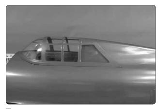
■ 8. Now is the time to securely install a pilot before gluing the canopy on. The pilot used is from Best Pilots. Wash the canopy in warm water, and then, dry it off. Place the canopy on the fuselage. Be certain it is centered from side-to-side and mark the outline on the fuselage. As before, prick holes in the covering just inside the outline. Use canopy glue to attach the canopy on the fuselage.
