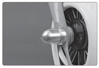
☐ 7. Secure the spinner cone to the spinner adapter with a 10-32 x 1" socket head cap screw (not included).
