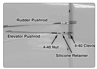
☐ 2. Thread a 4-40 nut, threaded clevis and a silicone clevis retainer, 12 turns, onto both elevator pushrods and the rudder pushrod.
