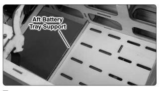
☐ 3. Glue the aft battery tray support to the battery tray and the fuselage sides.
