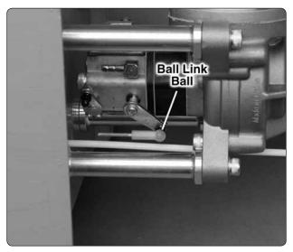
☐ 14. Thread the nylon ball link socket 14 turns onto the second 2-56 x 1" [25.4mm] threaded rod. Attach the ball link socket to the ball link ball on the throttle arm.
