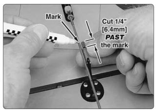
□ □ 3. Install the metal solder clevis in the second hole from the end of the control horn. Center the aileron servo and aileron. Mark the pushrod where it meets the solder clevis. Remove the pushrod and the solder clevis and cut the pushrod 1/4" [6.4mm] *past* the mark. Solder the solder clevis to the pushrod using the techniques described in the following **Hot Tip**.
