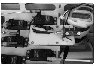
$\Box$  5. Cut off ½" (12.7 mm) from the threaded end of the 2-56 x 6" (152 mm) metal pushrod. Thread the nylon ball socket on the pushrod. Snap the ball socket onto the ball link ball on the retract control valve. Mark the pushrod where it crosses the servo arm and make a 90 degree bend at the mark. Install the pushrod in the servo arm and install a nylon Faslink. Cut the pushrod 1/8" (3 mm) past the top of the Faslink.
