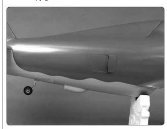
☐ 2. Glue the two innercooler exhaust doors in the two cutouts in the aft end of the fuselage.
