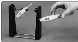
☐ 1. Carefully balance the propeller and any spare propellers. An unbalanced propeller can be the single most significant cause of vibration that can damage
