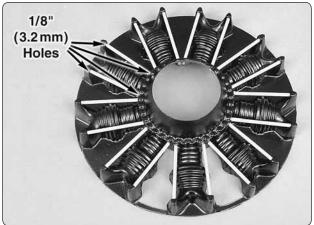
☐ 10. Drill 1/8" (3.2 mm) holes in the bottom of the rocker arms and in the crankcase as shown. Glue the eighteen aluminum tubes in the holes. Note that the aluminum tubes will need to be shortened if installed in the dummy engine used with the electric motor.
