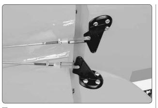
□ 3. Mount the control horns to the elevators and the rudder. Follow the same procedure used for the ailerons, by drilling 3/32" [2.4mm] holes and using #4 x 1/2" [12.7mm] sheet metal screws. Attach the elevator clevis in the third hole from base of the control horn. Install the rudder clevis in the second hole from the base of the control horn. Don't forget to harden the holes with thin CA after first installing, then removing the screws.
