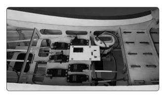
☐ 1. Test fit the retract servo tray in the fuselage. It should fit between the rudder and throttle servo. Drill
