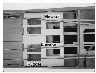
☐ 1. Hold your engine, inverted, up to the firewall. Determine which side the throttle and choke is on. Insert the three 4-40 x 48" (1220 mm) metal pushrods in the three outer pushrod tubes. The rudder pushrod should be installed on the opposite side as the throttle and choke.
