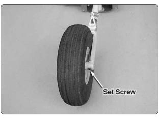
□ □ 2. Trim the axle that is included with the Robart retracts to 1-1/2" [38mm] long. File a flat spot at the end of the axle. Insert the axle through the included 5" [127mm] wheel and into the retract. Apply a drop of threadlocker to the 10-32 x 3/16" [4.8mm] set screw, included with the retract, and tighten the set screw onto the flat of the axle. Make sure that the wheel rotates freely.
