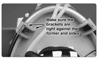
☐ 2. Position the two short cowl mounting brackets in the two bottom slots in the front of the fuselage.
