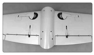
$\square$  8. Test fit the belly pan on the wing attaching it with four  $\frac{1}{4}$  - 20 x 2" (51 mm) nylon wing bolts.
