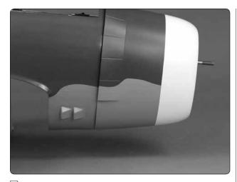
☐ 3. Glue the two oil cooler louvers to the forward lower fuselage following the same procedure used to install the turbocharger exhaust fairing.
