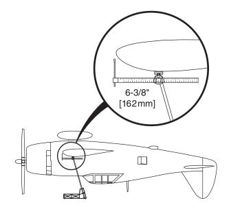
☐ 1. If using a Great Planes C.G. Machine, set the rulers to 6-3/8" [162mm]. If not using a C.G. Machine, use a fine-point felt tip pen to mark lines on the top of the wing on both sides of the fuselage 6-3/8" [162mm] back from the leading edge. Apply narrow (1/16" [2mm]) strips of tape over the lines so you will be able to feel them when lifting the model with your fingers.
