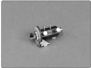
☐ 3. Assemble the retract control valve mount and install the retract control valve. Install a .080 ball link ball and .080 nut on the valve. Be sure to use a drop of threadlocker on the threads of the ball link ball.
