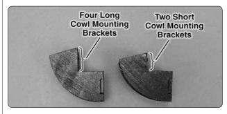
☐ 1. Note that there are four long cowl mounting brackets and two short cowl mounting brackets.
