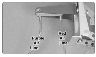
☐ 9. Connect a 24" actuator extension to the electric retractable tail gear or air lines to the pneumatic retractable tail gear.
