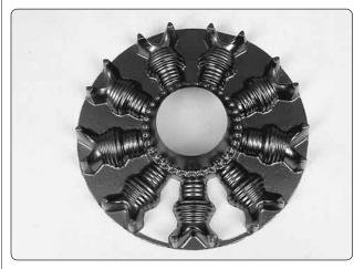
4. For installation with an electric motor, proceed to step 5. Cut out two openings between the cylinders and the center of the plastic radial engine. The center hole needs to be large enough to clear the drive washer of the gas engine. Proceed to step 10.
