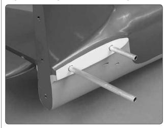
☐ 1. Test fit the two aluminum stabilizer tubes in the fuselage and slide the stabilizers on the tubes. The shorter tube goes in the front hole. If the aluminum tubes are too tight to slide through the holes, take a sharp hobby knife and gently scrape the inside of the holes. During the manufacturing process a small amount of resin or filler may be left behind in the hole.
