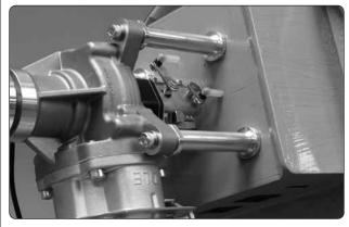
☐ 6. Snap a nylon ball socket onto both pivot balls. Center the choke and throttle arms and mark the firewall where the pushrods will need to pass through. Also mark the location where the fuel line will need to pass through the firewall.
