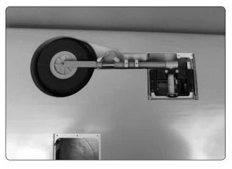
□ □ 3. Test fit the retract unit with the wheel into the wing. Position the retract so the wheel is centered in the wheel well. Adjust the strut position in the retract body as necessary to achieve the correct spacing all the way around the wheel.
