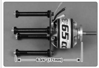
□ 5. Install the motor mount on the RimFire 65 following the instructions included with the XX-Large Stand Off Motor Mount. The front of the drive washer should be 6-3/4" (171mm) from the back of the stand off.
