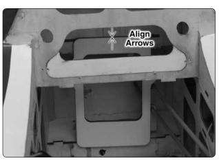
☐ 9. Glue the forward fuel tank support to the firewall, aligning the embossed arrows. The edge of the tank support should align with the two slots.
