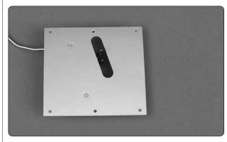
$\Box$  5. Drill 1/16" [1.6mm] holes through the blocks at the two hole locations on the top of the aileron servo hatch. Install two #2 x 3/8" [9.5mm] flat head sheet
