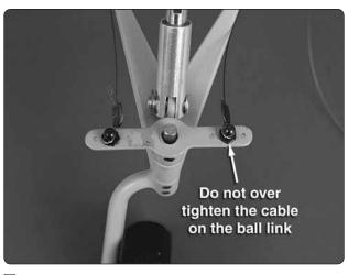
■ 8. Now pull on the long end of the cable to reduce the size of the first loop. Slip the loop over one of the ball link balls on the steering arm. Tighten the loop until it is small enough to remain secure on the ball, yet may still be pried off. Squeeze the swage with pliers. Connect the other cable to the other ball link ball the same way.
