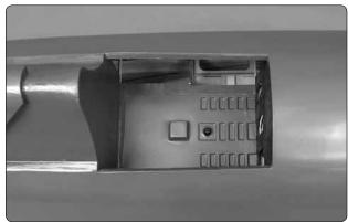
☐ 4. Trim the cockpit floor along the edge so that it lays flat. Use medium CA to glue the floor in the bottom of the cockpit. The floor should be positioned as far forward as possible. Drill a 1/8" (3.2 mm) hole through the control stick boot.
