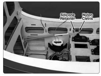
☐ 12. Thread a 2-56 x 1" [25.4mm] threaded rod approximately 3/8" [9.5mm] into the end of the white inner pushrod tube. Thread a nylon clevis 14 turns onto the end of the threaded rod. Slide a silicone clevis retainer over the clevis. Inset the white inner pushrod tube in the throttle's outer pushrod tube. Attach the clevis to the throttle serve arm.
