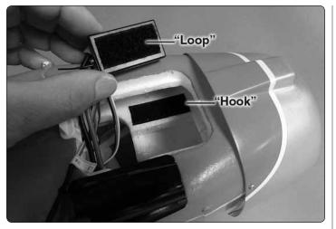
1. Apply a strip of the softer, "loop" side of the included double-sided adhesive-back Velcro® strip to your receiver (not included) and a strip of the rougher, "hook" side inside the fuselage where shown.
