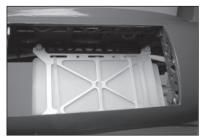
**111.** Remove the hatch from the top of the rear fuselage and set it aside in a safe location.
