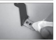
**15.** Test fit the aileron control horn. They should fit completely into the slot as shown. If they don't fit, use a file to enlarge the slot. Do not force the horn into place.
