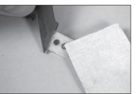
14. Use a paper towel and isopropyl alcohol to remove any oils or debris from the control horn. Prepare all four aileron control horns.
