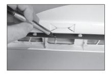
**57.** Use a felt-tipped pen to transfer the mark onto the flap and into flap control horn mounting area.
