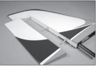
**72.** Install the control horn for the rudder using the techniques used for the aileron control horn.
