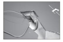
**85.** Retrieve the leads from the same location as the flap and aileron leads. Make sure to label the leads so they can be identified when assembling the model for flight.
