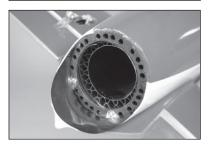
**127.** Space the exhaust tube equally between the sides of the fuselage. Secure the tube using four M3 x 12 self-tapping screws.
