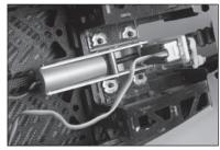
**94.** Route the leads for the retract and servo on opposite sides of the fuselage.
