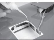
**42.** Secure the aileron servo cover using a #1 Phillips screwdriver and four M2 x 8 self-tapping screws.
