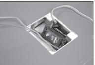
**53.** Guide the servo lead for the flap and aileron through the wing to the wing root.
