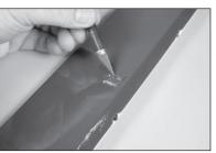
**13.** Lightly sand the area of the aileron control horns where they fit into the aileron. (The aileron control horns are the longest horns included.)
