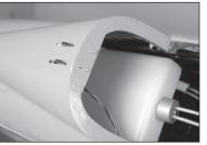
**147.** Connect the leads for the retract and brake inside the fuselage.
