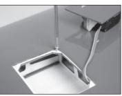
**41.** Apply 1–2 drops of thin CA in each hole to harden the surrounding wood. Allow the CA to fully cure before proceeding.
