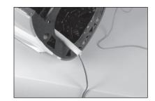
**123.** Slide the servo routing sleeves as far back as possible. Mark the sleeves at the bulkhead so the positioning can be checked before each flying session. Use tie wraps to secure the sleeves to the structure above the location for the thrust tube, so they don't come in contact with the exhaust tube during the operation of your model.
