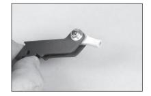
**20.** Slide the control horn base on the bottom of the control horn assembly.
