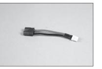
**82.** Use a hobby knife or sandpaper to sand a slight taper on each of the plugs on the leads (included with the retract module) that will connect to the receiver to the retract module.
