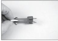
**21.** Fit the assembly into the slots in the aileron.
