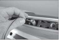
**119.** Wrap tape around the connection between the plug and string to make pulling the extension through the sleeve easier.
