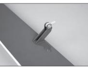
**22.** Place low-tack tape around the control horn base. This will help keep excess epoxy off the aileron.
