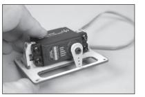
**34.** When connecting the clevis to the servo arm, use the hole that is 5/8 inch (16mm) from the center of the servo arm.
