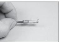
**44.** Remove the ball from the aileron control horn. Assemble the linkage so the length is  $3^{3}/_{4}$  inches (95mm).
