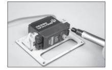
**30.** Remove the servo and use a pin vise with a 1/16-inch (1.5mm) drill bit to drill the four servo mounting holes.
