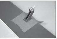
**23.** Remove the assembly and mix 1/2 ounce (15ml) of 30-minute epoxy. Apply epoxy in the control horn slots.
