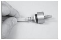
108. Use a wire tie to secure the fuel line to the clunk.
