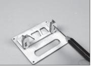
**31.** Thread a servo mounting screw into each hole, then remove the screws.
