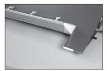
**67.** Attach the servo cover to the wing using four M2 x 8mm self-tapping screws.
