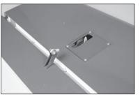
**43.** Slide a silicone retainer on the metal clevis. Thread the clevis on the 70mm threaded rod (on the end with the nut) until the end of the threaded rod is visible between the forks of the clevis.
