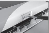
**61.** Place 2–3 drops of thin CA in each hole. Allow the CA to fully cure before proceeding.
