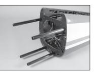
**138.** Prepare the five screws that secure the forward fuselage to the rear fuselage by sliding a tapered washer on an M4 x 20 socket head cap screw.
