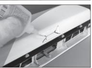
**62.** Secure the flap control horn to the flap using two M3 x 14 self-tapping screws and a #1 Phillips screwdriver. Note the orientation of the flap control horn.
