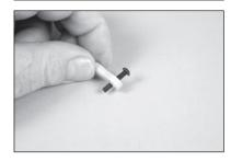
**48.** Remove any tape from the wing and flap. Assemble the flap linkage using two prepared ball ends and an 80mm threaded rod. Thread the ball ends equally on the threaded rod until the length is approximately  $4^{1}/_{4}$  inches (108mm).
