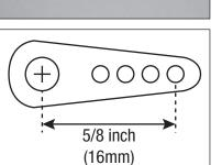
**52.** Install the flap servo with the output forward. Use the hardware included with the servo.
