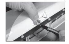
**59.** Place the horn aside. Use a 1/16-inch (1.5mm) drill bit to drill the two holes for the flap control horn mounting screws.
