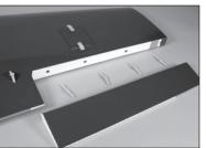
**12.** Lightly rub a finger over the bottom of the aileron to locate the mounting slots for the aileron control horns. Use a hobby knife and #11 blade to remove the covering for the aileron control horns.
