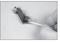
**25.** Fit the assembly into the aileron. Use a paper towel and isopropyl alcohol to remove any excess epoxy. Allow the epoxy to cure, then remove the tape.
