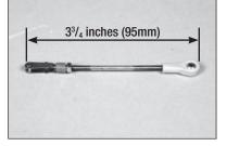
**45.** Attach the ball end to the control horn, then the clevis to the servo arm. With the radio system on and the aileron servo centered, adjust the linkage to center the aileron. Once adjusted, slide the silicone retainer over the forks of the clevis.
