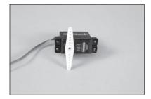
**50.** Place the flap servo into position with the output forward. Use side cutters to remove the excess servo arm extending out of the servo opening.
