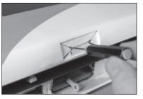
**60.** Use a #1 Phillips screwdriver to thread an M3 x 14 selftapping screw into each hole. Remove the screws before proceeding.
