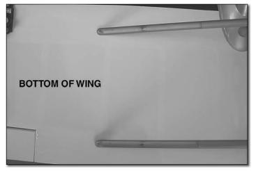
☐ 4. After installing the struts to the fuselage turn the airplane upside-down. Align the struts on the wing making sure that the strut rests on the wood sheeting, not the open wing structure. Carefully drill a 1/16" [1.6mm] hole in the **bottom** of the wing but **do not drill through the top of the wing!**
