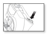
**NOTICE:** If the aircraft is upside down when the Panic Recovery trigger is pressed, sufficient altitude is required for the aircraft to return to straight and level flight.
