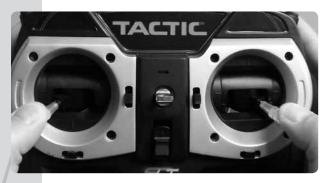
1. With the Tx power switch off, move the right stick to the bottomright corner, the left stick to the bottom-left corner, and hold in these positions.
