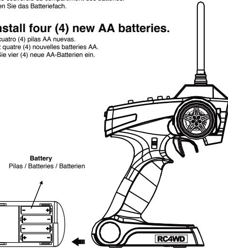
**Warning: Please replace batteries when the power indicator blinks or the buzzer beeps.**
