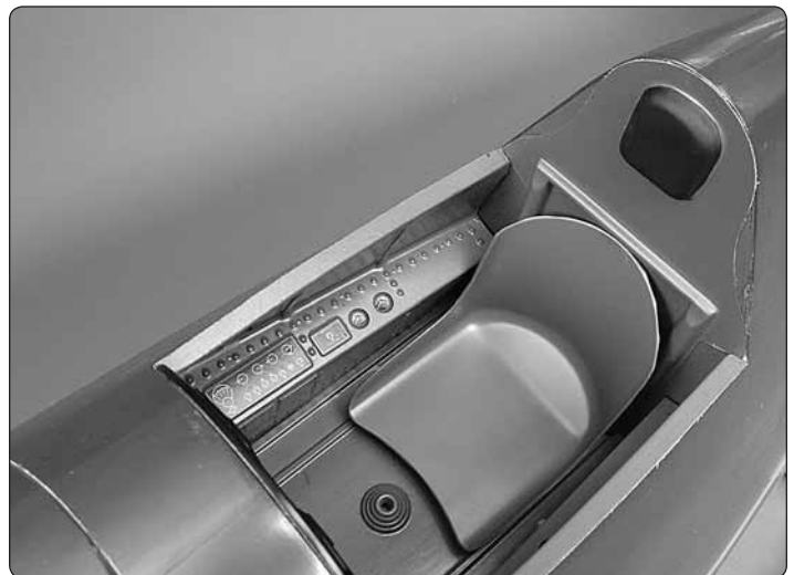
❑ 10. Use sandpaper to rough up the bottom of the seat. Glue the seat on top of the pedestal. Note: If a pilot will be installed, test fit it in the seat and the cockpit before gluing the seat on the pedestal.
