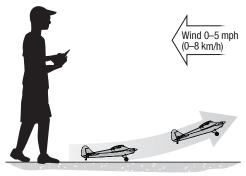
Gently pull back on the elevator stick to lift off the ground.
