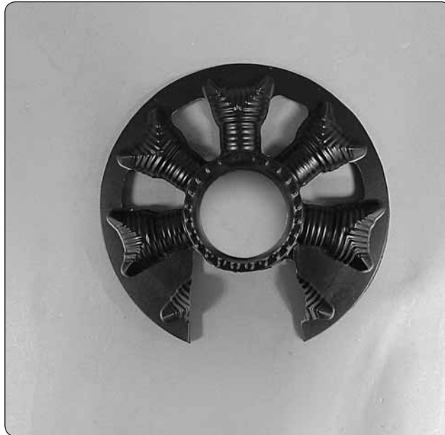
□ 16. Place the dummy engine in front of the engine. Using the engine as your guide, make reference marks on the dummy engine where the engine cylinder head is and cut away that area from the dummy engine.
