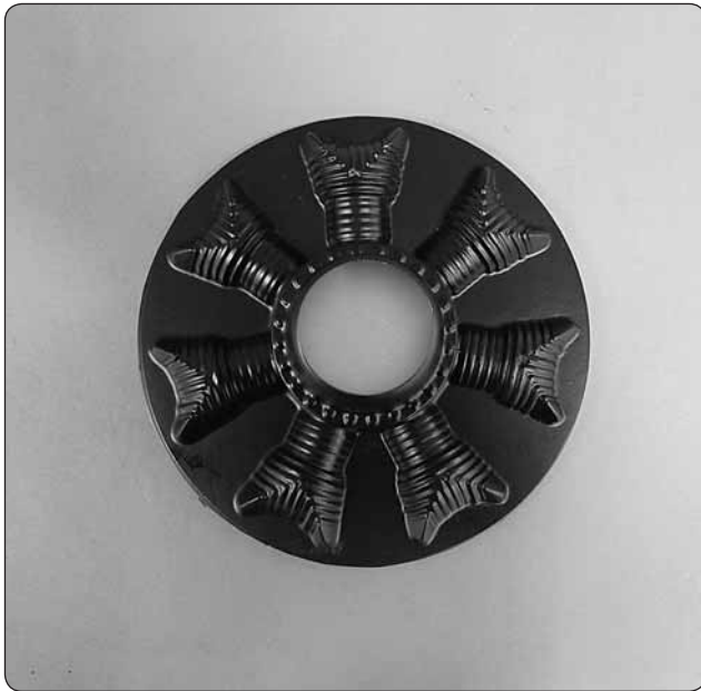
□ 14. Using a high speed rotary tool remove the center from the dummy engine.
