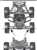
\*Front arms inner and outer hinge pins should be in a imaginary horizontal line when ride height is set.
