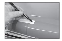
→ When flying in higher temperatures, the cowling can be modified to force more air over the engine. Trim the cowling to provide an additional air inlet to the engine.
