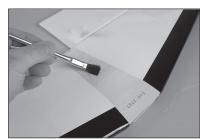
**72.** Mix 3/4 ounce (25ml) of 30-minute epoxy. Use an epoxy brush to apply epoxy to the exposed wood on the top of the stabilizer.
