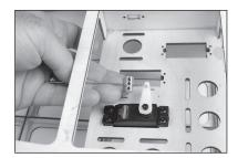
→ The arm will attach perpendicular to the servo centerline. Check this alignment before attaching the pushrod and removing any of the servo arms.
