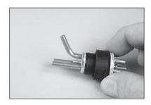
**152.** Secure a 12-inch (300mm) fuel line to the fill, vent and clunk tubes of the fuel tank. Tie wraps can be used to secure the fuel lines as an alternative to wire ties on the outside of the fuel tank.
