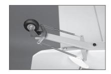
91. Remove the clevis and nut from the two 23<sup>5</sup>/<sub>8</sub> inch (600mm) pushrods. Slide both pushrods through the tubes in the fuselage. The pushrods will exit under the stabilizer.
