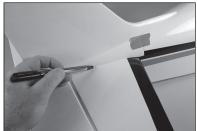
**69.** Remove the rudder and hinges from the fin. Place the fin on the stabilizer and trace the outline on the top of the stabilizer using a felt-tipped pen.
