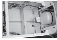
**157.** Use hook and loop tape and a hook and loop strap to secure the ignition battery at the front of the fuel tank tray.
