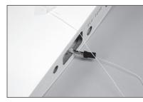
**29.** Secure a 9-inch (225mm) servo extension to the servo lead using a commercially available retainer (Servo Connector Clips, SPMA3054).
