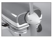
**168.** Glue the exhaust on the left and right sides of the cowling using a flexible adhesive.
