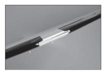
**70.** Trace the outline on the top of the fuselage using a felt-tipped pen.
