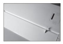
**21.** Once the CA has fully cured, gently pull on the wing and aileron to make sure the hinges are secure.
