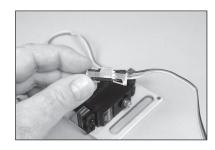
**34.** Secure the aileron servo cover using a #1 Phillips screwdriver and four M2.5 x 10 self-tapping screws.
