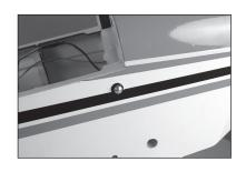
**156.** Use a sanding block and medium grit sandpaper to sand the bolt flush with the top of the tray so it doesn't damage the fuel tank when it is mounted to the tray.
