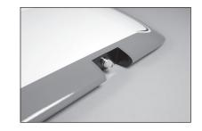
**45.** Move the control at the transmitter to the raised flap position. Adjust the throw percentage of throw at the radio to align the flap with the trailing edge of the wing at the root.
