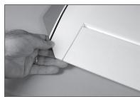
**22.** Break in the hinges by flexing the control surface through its range of motion in both directions.
