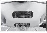
167. Remove the cowl and use a pin vise and 1/8-inch (3mm) drill bit to drill the four holes for the cowl mounting screws.
