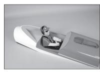
**175.** Use canopy glue to attach the canopy to the cockpit. Use low-tack tape to hold the canopy in position until the adhesive fully cures.
