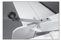
89. When attaching the linkage to the servo arm, use the hole that is 13/16 in (21mm) from the center of the servo horn. This hole will need to be enlarged using a pin vise and 5/64-inch (2mm) drill bit.
