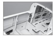
**133.** Remove the engine from the mounts. Use a drill and 11/64-inch (4.5mm) drill bit to drill the holes for the engine mounting screws.
