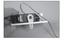
**41.** When attaching the linkage to the servo arm, use the hole that is 13/16 in (21mm) from the center of the servo horn. This hole will need to be enlarged using a pin vise and 5/64inch (2mm) drill bit.
