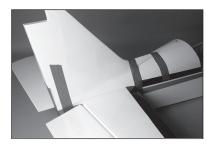
**79.** Use a drill and 1.5mm drill bit to drill the two holes for the tailwheel arm mounting screws.
