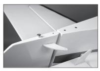
**76.** Locate the control horn marked "R" for the rudder. Use 5-minute epoxy to glue the rudder control horn in position. Allow the adhesive to fully cure before proceeding.
