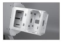
**121.** Attach the motor box to the firewall using four M4 blind nuts, four M4 washers and four M4 x 20 socket head cap screws. Use threadlock on the blind nuts to prevent them from vibrating loose.
