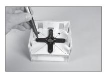
**111.** Remove the mount and drill the holes for the motor mounting screws using drill and 7/32-inch (5.5mm) drill bit.
