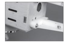
**132.** Use a felt-tipped pen to mark the location for the four engine mounting bolts on the engine mount.
