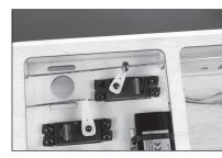
→ When mounting the throttle servo on the opposite side as shown in the manual, a support must be fabricated to support the pushrod tube for the throttle pushrod to operate properly
