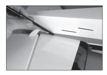
Check the position of the stabilizer repeatedly during the curing process to make sure it has not moved.
