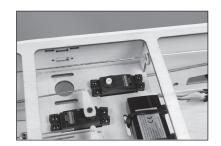
143. Move the carburetor and servo to the low-throttle position and tighten the setscrew securing the pushrod to the connector at the servo. Use side cutters to trim the excess wire. Check the operation of the carburetor using the radio system. Make any adjustments necessary to fully open and close the carburetor using the radio system.
