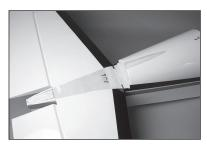
**67.** Mix 3/4 ounce (25ml) of 30-minute epoxy. Use an epoxy brush to apply epoxy to the exposed wood on the bottom of the stabilizer.
