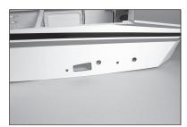
**61.** Stand back 8-10 feet (2-3 meters) and check that the stabilizer is aligned with the wing. Lightly sand the stabilizer saddle on the fuselage to correct any misalignment.
