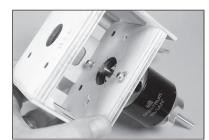
118. Slide the plate forward. Use a paper towel and isopropyl alcohol to remove any excess epoxy. Use tape to hold the sides of the motor box tight against the plate until the epoxy fully cures.
