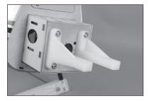
**135.** Use a drill and 5/32-inch (4mm) drill bit to drill the hole for the throttle pushrod.
