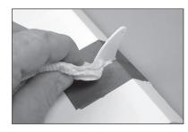
15. Fit the flap into position on the hinges.
