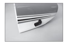
→ Trim the cowling around the engine, then use light plywood or foam board to create a baffle that will direct air directly over the engine.
