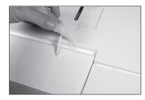
**24.** Use a toothpick or hobby knife with a #11 blade to puncture the aileron servo cover for the mounting screws.
