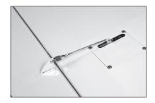
**44.** With the flap servo centered using the radio system, adjust the linkage to achieve the 1 inch (25mm) mid-flap throw.
