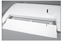
Use a rotary tool and 1/16-inch (1.5mm) drill bit to drill the location in the wing trailing edge and control surfaces marked in Step 1.
