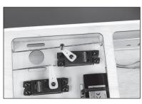
→ The servo tray has locations on either side of the fuselage for the throttle servo. Use the location that best suits the engine selected for your model.
