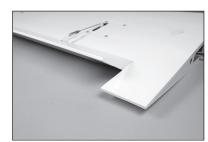
50. Use canopy glue to glue the landing light cover to the wing. Use low-tack tape to hold the cover in position until the adhesive fully cures.
