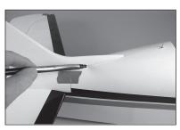
**66.** Use a hobby knife with a #11 blade to carefully cut the covering at the trailing edge when the stabilizer comes into contact with the fuselage.
