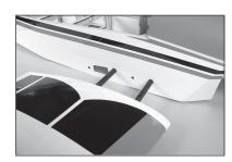
62. Measure from each wing tip to each stabilizer tip. Adjust the stabilizer so the measurements are the same for both sides.
