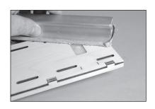
**122.** Remove the plate from the fuselage to allow cooling air to enter the fuselage.
