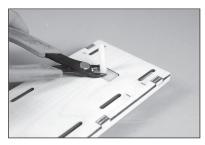
**129.** Slide the tray with the battery into the fuselage. The tray is then secured at the rear using a 1/4-20 nylon bolt.
