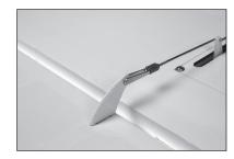
**42.** Locate the linkage for the flaps. With the clevis removed, the linkage will measure 3<sup>1</sup>/<sub>2</sub> inches (90mm).
