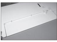
Use a paper towel and isopropyl alcohol to remove any excess epoxy.
