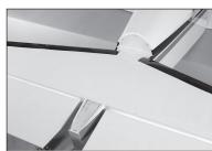
**56.** Use a hobby knife with a #11 blade to remove the covering for the two wing bolts and the opening for the servo leads on both sides of the fuselage.
