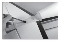
**73.** Use an epoxy brush to apply epoxy to the fin mounting surface.
