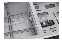
99. Center the rudder servo using the radio system. Remove the clevis and nut from the rudder pushrod and slide it into the rudder pushrod tube in the fuselage. Attach the servo arm to the servo. Remove any arms from the servo horn the will interfere with the operation of the servo and linkage using side cutters.
