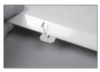
Apply epoxy to the area of the control horn that fits into the slot. Apply epoxy to all the surfaces of the control horn that fit into the control surface.
