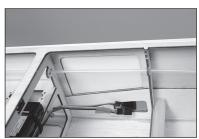
134. Mark the location of the throttle pushrod on the firewall using a sharpened wire or felt-tipped pen. Remove the engine from the mount.
