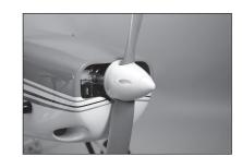
**166.** Once aligned, mark the locations for the cowl mounting screws on the cowl using a felt-tipped pen.
