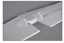
**71.** Use a hobby knife with a #11 blade to carefully cut the covering 1/8 inch (3 mm) inside the line drawn on the top of the stabilizer and fuselage to remove the covering. Use care not to cut into the underlying wood, weakening the stabilizer or fuselage.
