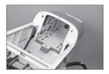
**155.** Remove the tray from the fuselage and use side cutters to remove the excess bolt from the upper side of the tray.
