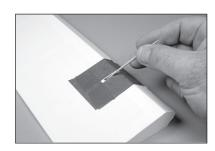
**13.** Fit the hinge in the hinge slot. Align the slot in the hinge with the hole in the wing. Install the hinges for the aileron and flap.
