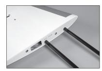
**60.** Place the stabilizer in position. The control horn will be on the bottom of the elevators when installed.
