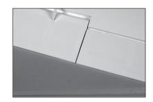
**19.** Finally, check the gap between the wing and flap at the wing root. Adjust the position of the aileron and flap so all three gaps are equal.
