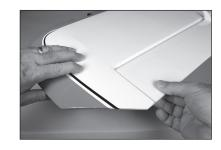
**17.** Check the gap between the aileron at the wing tip.
