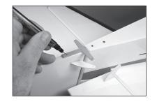
74. Position the fin back on the fuselage. Use a paper towel and a small amount of isopropyl alcohol to remove any excess epoxy from the fuselage and stabilizer before the epoxy fully cures. Use low-tack tape to hold the fin secure while the adhesive fully cures. Allow the epoxy to fully cure before proceeding.
