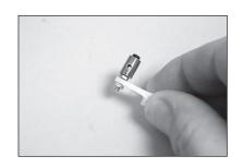
**142.** Center the servo using the radio system and install the servo arm on the servo, perpendicular to the servo center line
