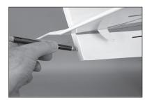
**80.** Thread an M2.5 x 10 sheet metal screw into each hole using a #2 Phillips screwdriver
