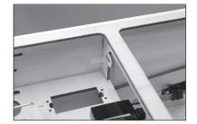
139. Slide an M4 washer on each M4 x 30 machine screw, then place an M4 locknut on each screw. Use a #2 Phillips screwdriver and 7mm hex driver to tighten all four screws, securing the engine to the engine mount.
