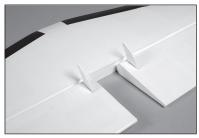
**53.** Use a small piece of low-tack tape to hold the elevators in alignment with the stabilizer for the next few steps.
