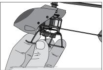
Hold the bottom of the Scout CX as shown to keep from damaging the circuit board.
