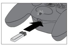
Replace transmitter batteries when the transmitter sounds an alarm (multiple beeps) while flying. Also, replace the batteries if flight battery charging takes longer than 30 minutes AND the charge LED remains solid.
