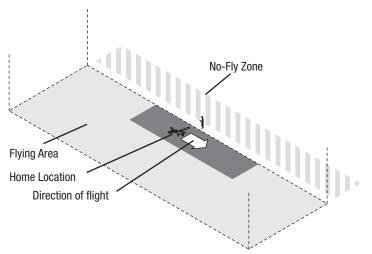
In this example *right aileron* would be applied to set the flying field side.
