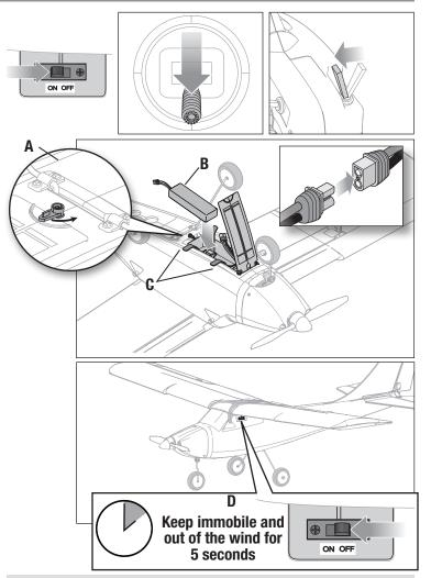
**CAUTION:** Always disconnect the Li-Po flight battery from the aircraft receiver when not flying to avoid over-discharging the battery. Batteries discharged to a voltage lower than the lowest approved voltage may become damaged, resulting in loss of performance and potential fire when batteries are charged.
