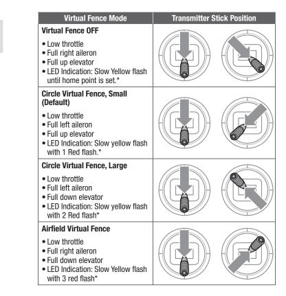
LEDs are located in the center of the front windshield of the aircraft. \*A purple flash will follow all mode indicators to indicate LAS is installed.
