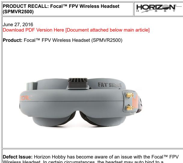
**Defect Issue:** Horizon Hobby has become aware of an issue with the Focal<sup>™</sup> FPV Wireless Headset. In certain circumstances, the headset may auto bind to a Spektrum<sup>™</sup> receiver and take control of functions assigned to Channels 6 or 7. If the Spektrum<sup>™</sup> receiver is installed in an aircraft and these channels are set to arm the motor, it may cause an uncommanded engagement of the aircraft's throttle. This may lead to property damage and injury.
