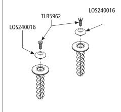
**Body Mounting Option 3:** Hard mounted body. Body is secured to the body mounts with screws and body buttons.
