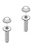
**Body Mounting Option 1:** Screw on style body mount uses a screw top to secure body to body mount post.
