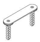
**Body Mounting Option 2:** Hook and Loop body mount. Use the cross bar mounted to the body mounts to apply hook and loop so you can mount your body without drilling any holes.
