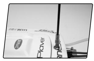
4. For added security, you can use a small piece of silicone tubing to hold the antenna in place.
