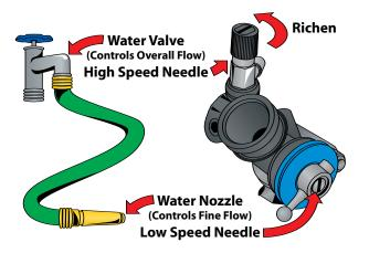
is increased, the low-speed needle is pulled completely away from the needle seat leaving it fully open. At that point, fuel metering is entirely controlled by the high-speed needle. Again, using our water hose example, when the spray nozzle at the end of our garden hose is fully open, then the main water valve can be used to adjust how fast the water flows.
