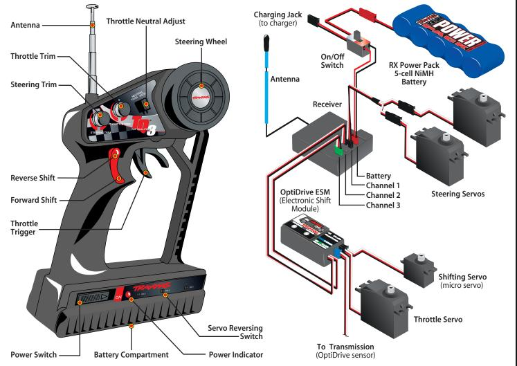
The OptiDrive ESM is designed to adapt and work with aftermarket three channel radio systems (see page 15). Learn terms related to the TRX 3.3 Racing Engine beginning on page 20.
