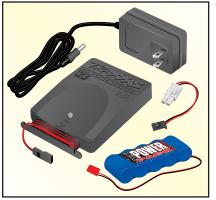
To power the radio system in the truck, your Revo is equipped with the RX Power Pack, a rechargeable 5-cell nickel metal hydride (NiMH) battery pack. The RX Power Pack must be fully charged before running the truck. The supplied TRX Power Charger is a peakdetecting unit that will charge the supplied RX Power Pack in about one hour. The peak-detection
