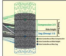
adjustments. The suspension sag and spring pre-load should be readjusted anytime the springs are removed and/or replaced.
