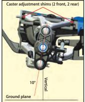
caster angle of the front suspension can be adjusted from 5° to 15°. Adjust the caster by positioning the caster adjustment shims on the upper control arms of the front suspension as shown in the table below:
