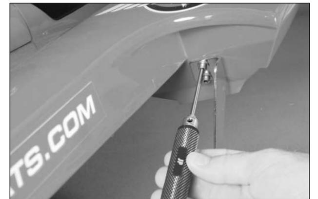
5. Carefully attach the turn fin onto the right sponson as shown and tighten the hex screws with a 3mm hex driver.
