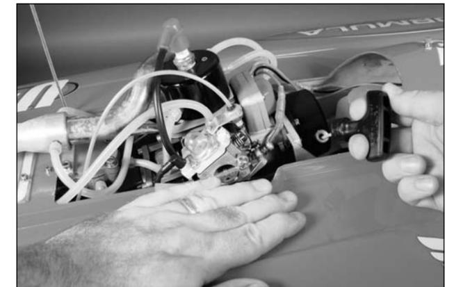
With an assistant holding the boat to the boat stand and bracing the engine with one hand, pull the starting cord briskly several times. Once the engine fires (begins to start), open the choke. Prolonged choking will flood the engine with fuel. See Section 15: Troubleshooting Guide to correct the flooding condition.
