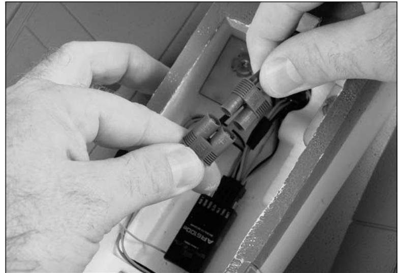
**Note:** Make sure to be clear of the propeller when connecting the battery in case the motor starts unexpectedly.
