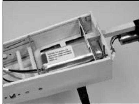
**Hint:** You may use a piece of hook and loop strapping around the battery to help secure it in position.
