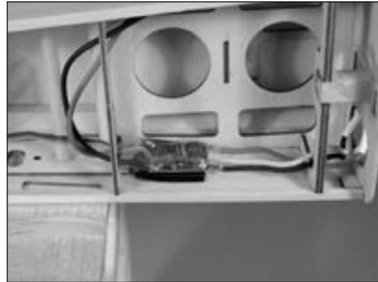
**Note:** When mounting the EFLA311 ESC, a 35mm x 20mm x 7mm balsa block is required to space the ESC away from the fuselage side.
