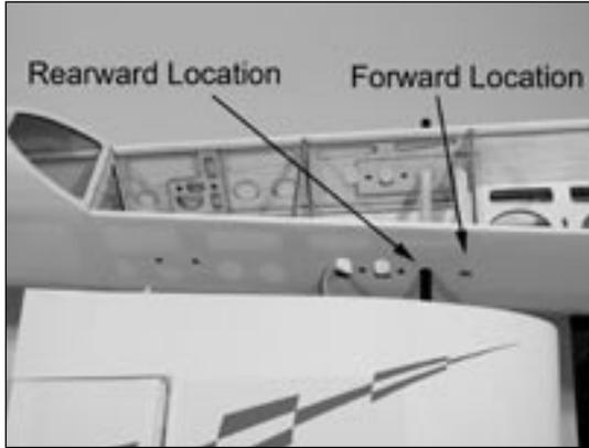
**Note:** There are two locations for the wing tube in the fuselage. Use the rear hole (rearward wing location) at this time. Details regarding the different wing positions are described under the Center of Gravity section.
