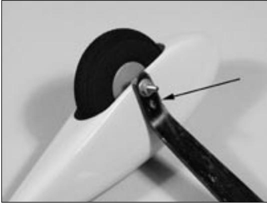
**Note:** Use threadlock on both nuts to prevent them from loosening during flight.
