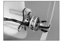
prop. Hook the rubber O-ring to one of the countersunk screws. Stretch it across the hub of the prop and hook it onto the other countersunk screw to retain the propeller. Use thread locking compound on all screw threads.
