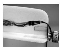
motor. If it does not rotate correctly, unplug the micro 3-pole connector and rotate it 180°. This will reverse the motor rotation. **Note:** Do not install the prop for this step.
