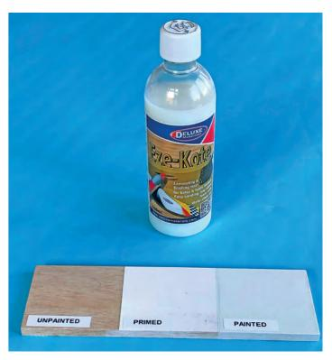
Having sanded the wing, Andy tested it using Halfords White Primer and his chosen paint, Halfords Spray Ford Diamond White. Eze-Kote has good compatibility with most white car primer paints. If you're in doubt always check by testing the primer and paint topcoat before committing it to the model.
