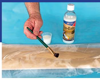
Eze-Kote is then brushed through the glass fibre fabric. Any unused Eze-Kote can be returned to its container.
