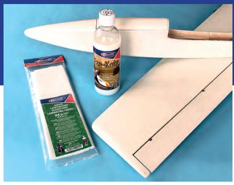
A second coat of Eze-Kote is applied after the glass cloth has been trimmed. After sanding and further filling, if required, the model is ready for painting.
