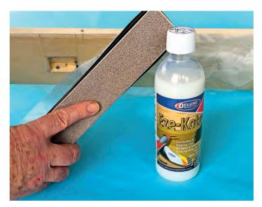
Excess fabric is effortlessly trimmed away using Perma-Grit sanding block or 320 grit paper.
