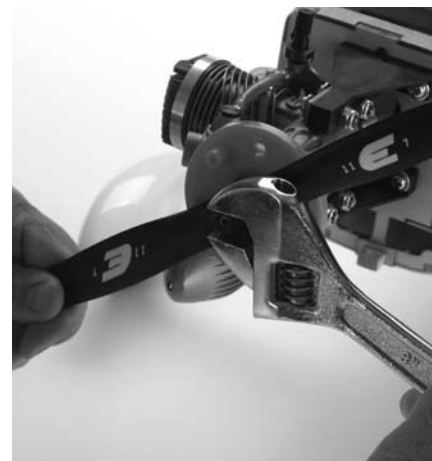
Securely tighten the prop nut using a wrench.
